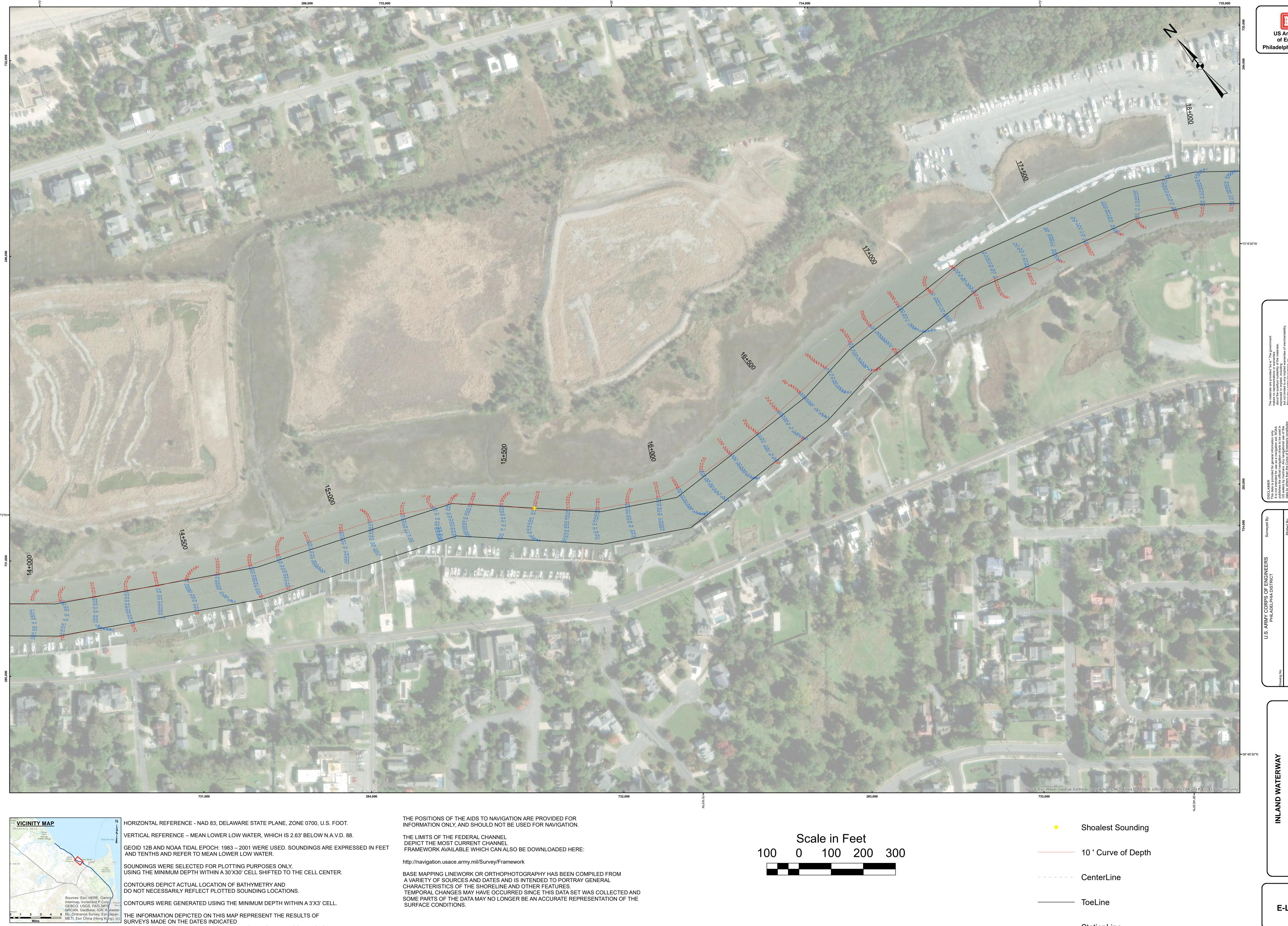
CONTOURS WERE GENERATED USING THE MINIMUM DEPTH WITHIN A 3'X3' CELL.
